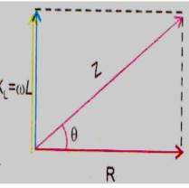
The voltage will lead the current by a phase  $\theta = \tan^{-1} \left(\frac{X_L}{R}\right) = \tan^{-1} \left(\frac{\omega L}{R}\right)$ .
