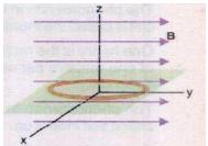
**iii.** When the coil is rotated about z-axis, no change of flux takes place through the coil, hence induced emf and current will be zero.
