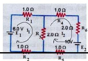
assigned current to both loops in clockwise direction.
