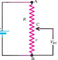
term Ir (voltage drop across internal resistance) increases which decreases terminal potential difference.
