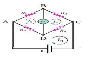
It consists of four resistances connected in the form of a bridge (mesh), a galvanometer, a battery and a switch. When the switch is closed and bridge is made to operate balanced condition by varying the known resistances, no current passes through the galvanometer and following condition is satisfied:-
