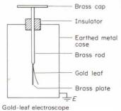
is brought near the brass cap (disc), it induces a negative charge on the surface
