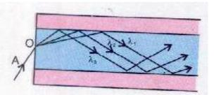
different paths across the core. The wavelength(s) which meet(s) the cladding at greater angle than critical angle, reach earlier at other end while the wavelength which meet the cladding at critical angle lags behind others. Hence, different component reach the other end at different times and signal received is distorted.
